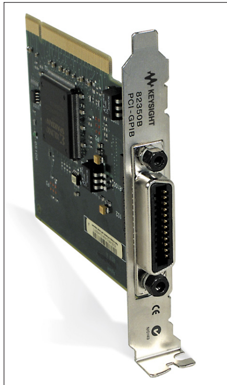
82350B PCI high-performance GPIB interface card
